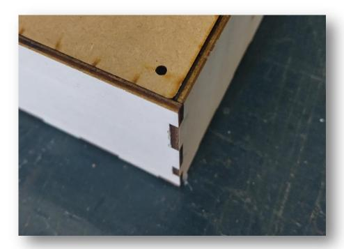
Using a 1mm drill bit drill four holes in the corners of the MDF panel backing. The MDF panel has four holes already cut, place the drill bit in the centre of these holes and drill into the square block beneath. These holes are to hold down the face of the mimic panel.
