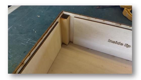
Now place the mimic panel MDF backing on top of the enclosure. Any button markings or text should go inside the enclosure so they are not visible from the outside.
