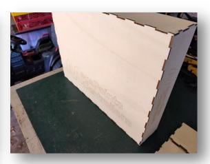
The enclosure comprises five outer pieces, the base and four sides and four inside lips that support the mimic panel backing MDF. Four corner pieces are also installed to accept the corner screws that will lock down the mimic panel as shown below.
