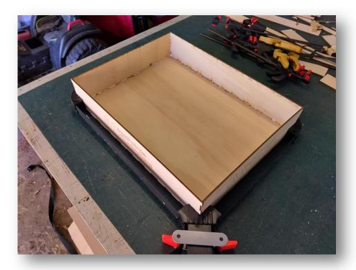
Turn the enclosure over and check the base is correctly seated against the sides. It may help to gently weight down the base.
