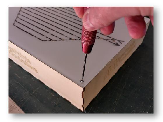
As a last step, decide where you would like your cables to exit the enclosure and drill a suitable hole.
