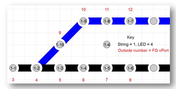
Add the corresponding FG vPorts (shown in red numbering) in the above diagram.
