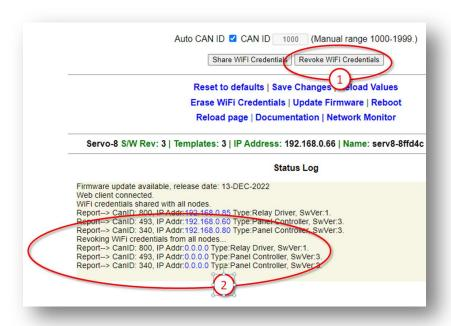
You will observe in the Status Log revocation messages. Each board will restart and show an IP address of "0.0.0.0" showing that it is not connected to any Wi-Fi network.
