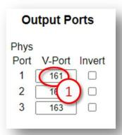
The Output Ports section of the Panel Controller (1 left) matches the Feedback V-Port of the Servo-8. It is this port that is listening for the event.
