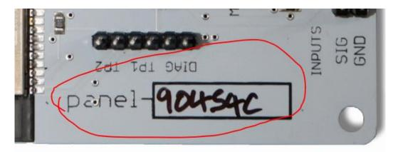
The device name is "panel-90454c". Use this name to connect to your device. In your browser address bar (not search bar or google search) enter "http://panel-90454c.local" and your network should locate the device for you. You won't need to enter the IP address again. In the above example substitute your devices name and serial number.
