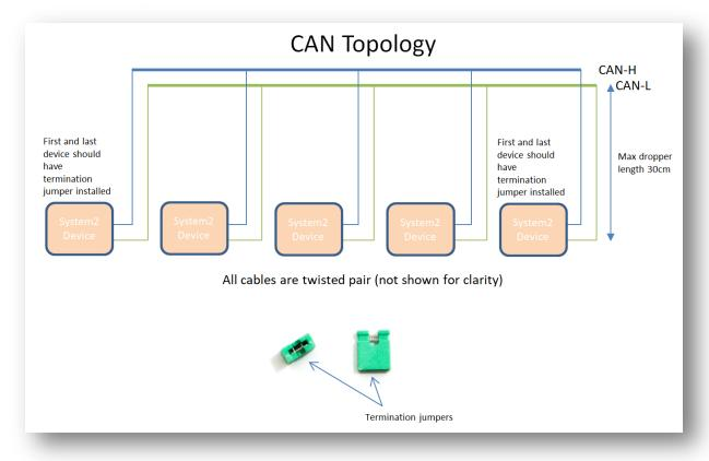
You can fit the termination jumpers to the first and last board on your network if not already fitted (see above two diagrams). The jumpers may have been pre-installed to all boards, remove all except the first and last System2 boards on the network.
