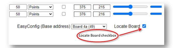
First, it will cause the flashing LED indicator on that board to flash rapidly. This helps locate and identify the board if you have multiple boards in one location.
