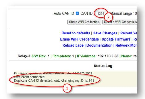
The CAN ID was automatically changed to an unused ID. When the board is rebooted or the web page refreshed the CAN ID field will update to the new value.
