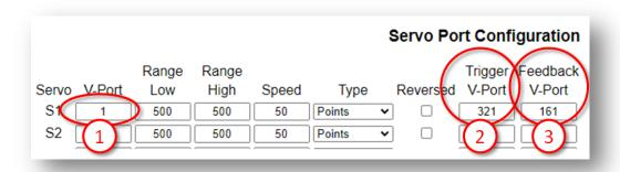
The V-Port (1) is 1 meaning channel S1 (servo 1) is listening for this address (V-Port).
