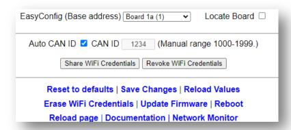
If a duplicate ID is detected and the address manually configured you will observe a message in the Status Log (example below) warning of the duplicate address and that auto change is disabled You need to manually reconfigure this.
