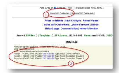
To revoke Wi-Fi access for all connected boards click the "Revoke WiFi Credentials" (1) button (see below):
