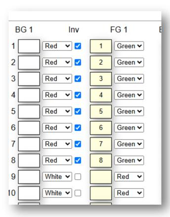
You should now have all RED LEDs indicating power failure (default setting).
