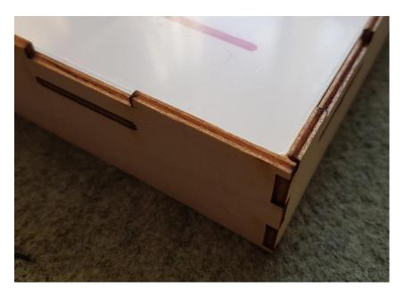
Carefully attach the top lip to the shell and check for correct fit.
