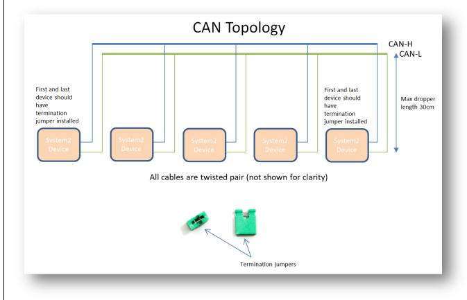
You can fit the termination jumpers to the first and last board on your network if not already fitted (see above two diagrams).
