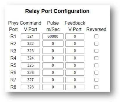
The Feedback V-Port will generate an event from the relay driver to indicate its position.
