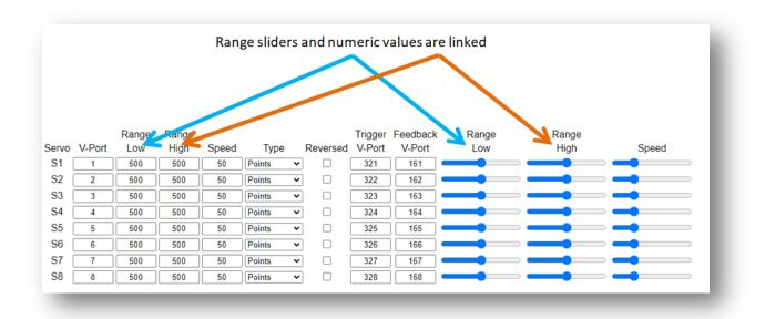
To dynamically adjust the opposite side first move the servo to the other side using your Panel Controller or other connected controlling device. This activates the live adjustment feature for that side. This avoids uncontrolled high speed servo swings before they are adjusted.
