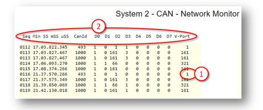
The V-Port the packet is intended for is decoded n the right column (1).
