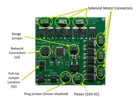
Power should be from a 2 Amp AC transformer at 16 Volts (30 VA). The power terminals (located at the bottom) have no polarity.
