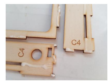
Work the lip into each edge piece carefully. Do not force any parts as this may break the component.
