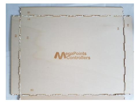
Use the elastic bands to secure the edges. Ensure all corners are fully interlocked and straight.
