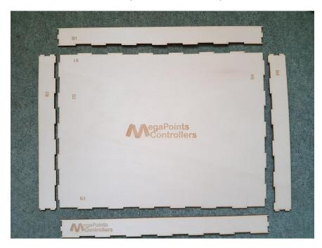
Turn the front panel over so the logo is facing down and apply wood glue to all facings. Don't forget the corners of the edge pieces.
