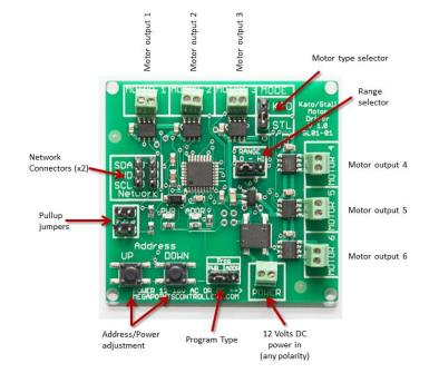
WARNING: Take care not to short circuit the motor terminals as this will result in damage to the output IC. Power should be from a 1 Amp (minimum) 12 volt DC power supply. The power terminals (located at the bottom) have no polarity.
