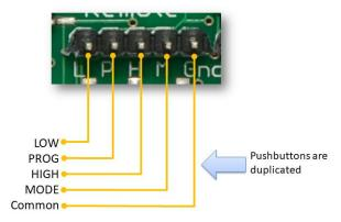
Use a pair of standard servo extension leads with plugs fitted or make your own to suit your requirements. Connect each of the left four cables to one connector of a pushbutton and connect the other pushbutton connector to each other and the common ground. Each pushbutton will mimic the four setup buttons on the board (*LOW, PROG, HIGH, and MODE*).
