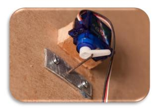
In the above image thin aluminium plate was used as a pivot for 1.2mm diameter piano wire connecting the servo to the points.
