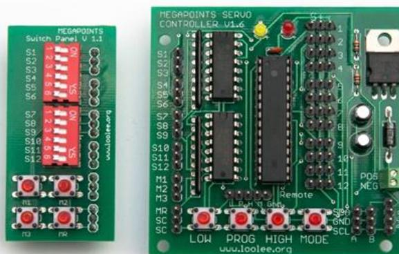
Pop-on switch board installed on Servo Controller.
