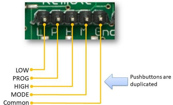
Use a pair of standard servo extension leads with plugs fitted or make your own to suit your requirements. Connect each of the left four cables to one connector of a pushbutton and connect the other pushbutton connector to each other and the common ground. Each pushbutton will mimic the four setup buttons on the board (*LOW, PROG, HIGH, and MODE*).
