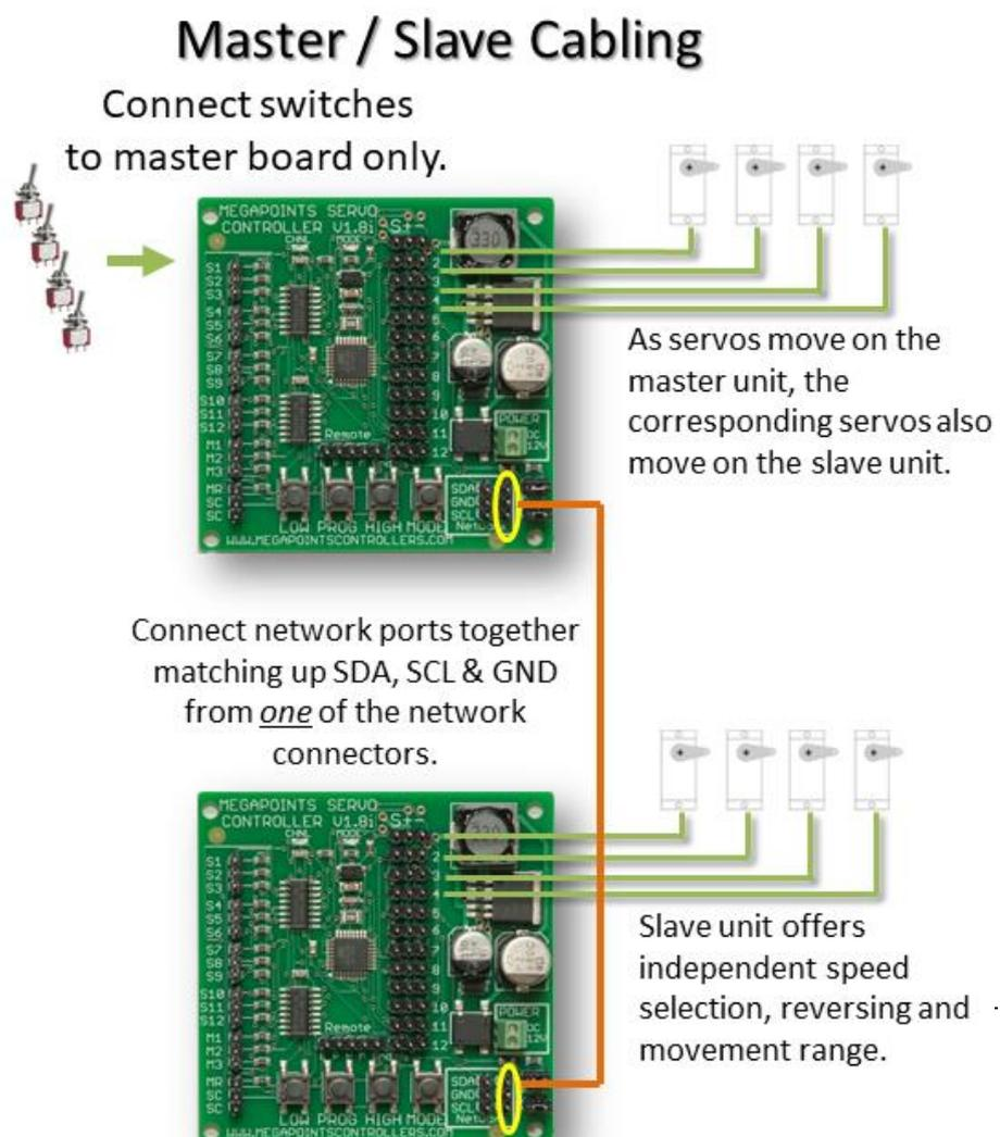
the track, the corresponding points are moved in synchronisation thus preventing the need for complex interlock mechanisms.
