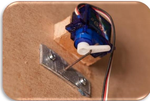
In the above image thin aluminium plate was used as a pivot for 1.2mm diameter piano wire connecting the servo to the points.
