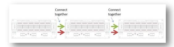
Additional LED expansion boards are daisy chained together using the short cables provided (see above).
