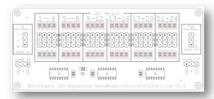
The LED expansion board (pictured above) provides an additional 48 LED outputs for 24 channels. Connect the "DATA IN" connector (top left side) to either "LED 1", "LED 2" or "Feedback" connectors taking care to match up the "DLC" pins using one of the short cables supplied.
